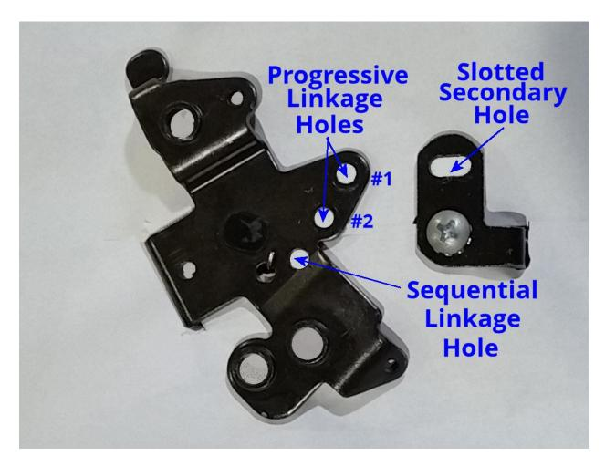
Detailed View of Primary and Secondary Linkage Levers
