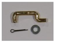
D. With the progressive link in place, replace the washer and secure with the new cotter pin. Ensure that the pin is bent adequately so that it will not fall out.
