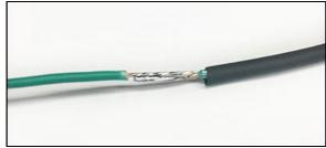
Soldered Connection w/ adhesive heat shrink
