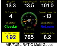
AIR/FUEL RATIO Multi-Gauge Engine below 160° F (NoLearn)
