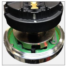
The relationship between the crank sensor, shutter wheel opening, and rotor in the picture above should match what is installed in your engine.
