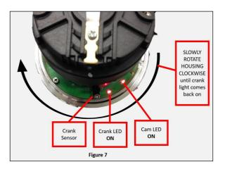
Turn the housing **clockwise** until the Crank LED comes back <u>ON</u> (**Figure 7**). Stop at this point. This will position the distributor close to where it needs to be. Install and snug the distributor clamp down at this point.
