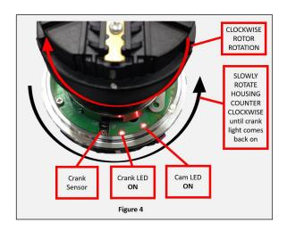
Then slowly turn the housing **counter-clockwise** until the Crank LED comes back <u>ON</u> (Figure 4). Stop at this point. This will position the distributor close to where it needs to be. Install and snug the distributor clamp down at this point.
