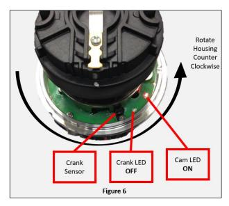
Slowly turn the housing <u>counter-clockwise</u> until the Crank LED goes <u>OFF</u> (Figure 6).
