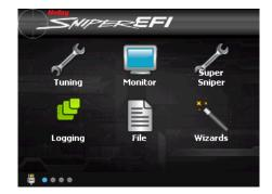
The Home screen contains icons which will navigate to different functional features of the 3.5" Touch Screen. These features will be discussed in detail throughout the main manual. The 3.5" Touch Screen will not display sensor parameters until a base calibration has been put in the unit using the Wizard.
