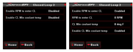
**Enable RPM to enter CL:** This setting is disabled by default. If an extremely large camshaft is used (specs only typically found on race camshafts), the overlap sometimes causes a "false lean" reading at low RPM. In these cases, it may be required to enable this function and put in a value of above idle RPM so the system operates open loop below this RPM setting.
