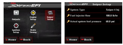
System Type: Change the calibration for different part numbers within the Sniper EFI Family
