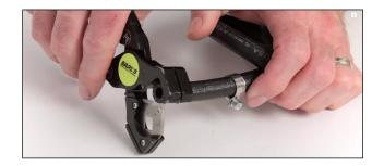
2. Install the fitting, by sliding the fitting into the hose. Make sure the hose seats flush with the fitting. (Figure 45-2)
