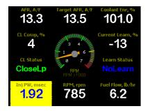
AIR/FUEL RATIO Multi-Gauge Engine below 160° F (NoLearn)
