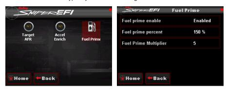
**NOTE:** This only injects fuel once at key-on, and will not do it again until the engine has run. This fuel prime occurs 2 ½ seconds after key-on. If you quickly turn the ignition key without waiting for 2 ½ seconds, the prime will not occur and it may take longer for the engine to start.
