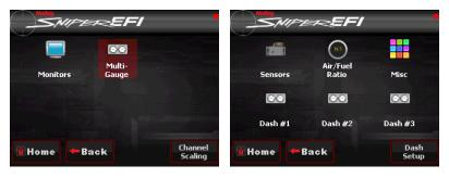
Below are an example of the Sensors Multi-Gauge and the Air/Fuel Ratio Multi-Gauge
