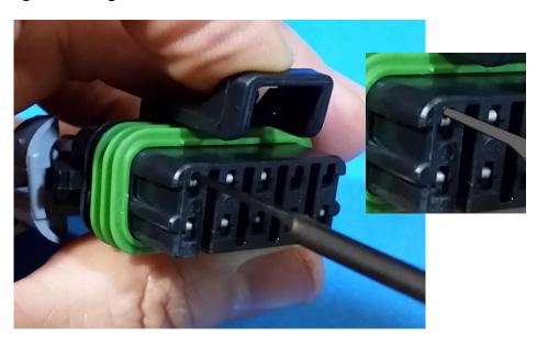
3. After you remove a terminal, replace it with one of the red cavity plugs included in the kit. The Sniper ships with two cavity plugs in the 10-pin connector so you can use these as a reference on how the should be inserted.
