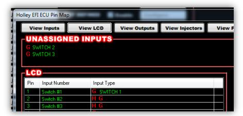
5. Select 'View Outputs' from the 'Pin Map' and drag the outputs to the whatever pin location the device was wired to.
