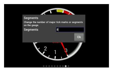
Note: Ensure the number of segments is matched up with the range you specify. E.g. If you choose 6 segments in a 0-8000 tachometer range, the scale markers will be at 0, 1333, 2667, 4000, 5333, 6667, and 8000. We would recommend using 4 or 8 segments instead.
