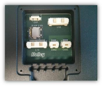
Figure 1. Slide door to the left to unlock
