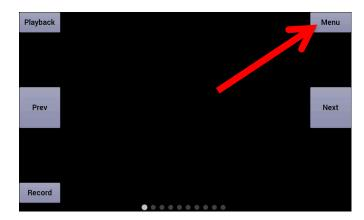
Pressing anywhere on a gauge screen will bring up the navigational buttons. To access the main menu choose 'Menu' in the upper right corner of the screen.
