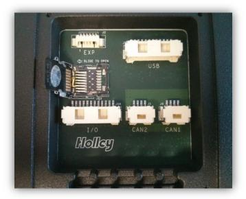
Figure 3. Insert micro-SD card
