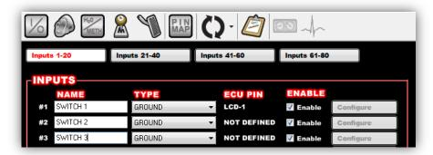
2. Create an output in the I/O screen and give it a name – in this example we have named them "Cooling Fan", "Elec Water Pump", and "NOS Bottle Htr". Once named, choose 'Configure' at the right of the screen.
