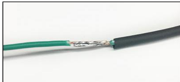
Soldered Connection w/ adhesive heat shrink
