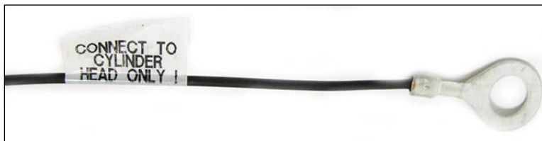
Figure 22 Coil Ground Wires
